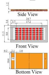
$VD-0808I-220W-1U-2A0+Case \ (Substrate\ 1=\underline{AIN}\ and\ Package\ U=\underline{2511},\ with\ water\ cooled\ case\ (unit:\ mm)$
