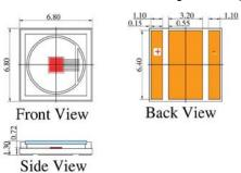
VD-0850I-006W-6K-2A0 with Substrate 6=Cu and Package K=T-mount (unit: mm)
