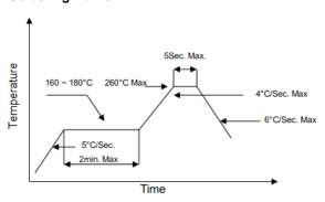
Note: Reflow soldering can be operated only one time. During the temperature ramp-up, no forces may be exerted on the diode which could deform or damage them. After soldering completed, please also do not process until the product temperature ramp down to room temperature.
