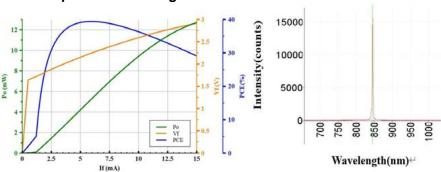
Note: 1. LIV graph was measured at 25 °C (left); power output, voltage and power conversion efficiency variation trend with changed operating temperature (right, normalized).
