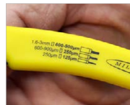
Convenient stripping guide printed on the tool handle.
