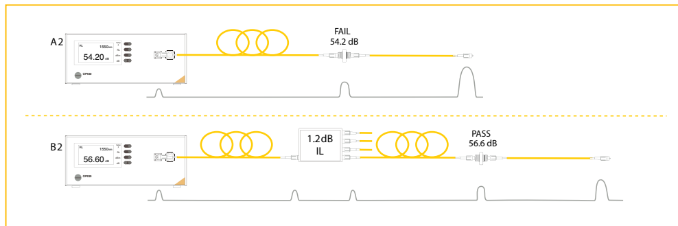
Figure 3: PC-PC connection degraded when traveling through same lossy system as in Figure 2 above
