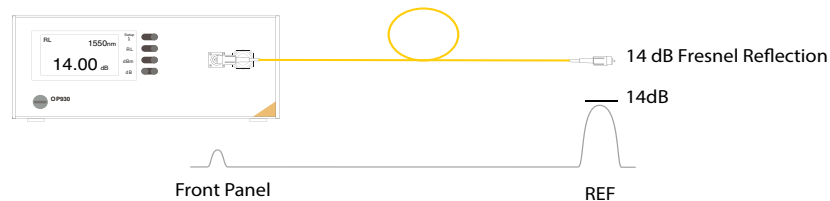
Figure 1: Typical OTDR-like trace for an open flat connector
