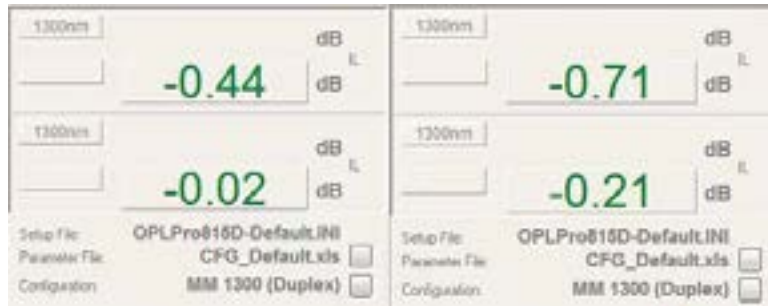
Figure 2: OPL-Pro live display for duplex cables
