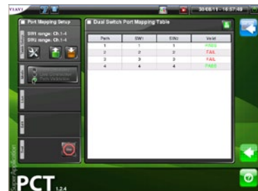
Port mapping (also called continuity or polarity testing) is enabled with two optical switches
