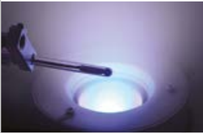
FIGURE 1. A Multipole Resonance Probe (MRP) monitors a plasma produced by an advanced plasma source (APS). (Copyright: INP – Leibniz Institute for Plasma Science and Technology)
