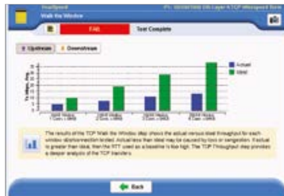
Figure 18. Failing Walk-the-Window results
