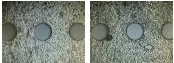
Similar to simplex cables, MTP reference cables must be free of dirt and damage to avoid creating excess insertion loss and return loss. Extension leads can prevent such damage from occurring to expensive MTP reference cables.
