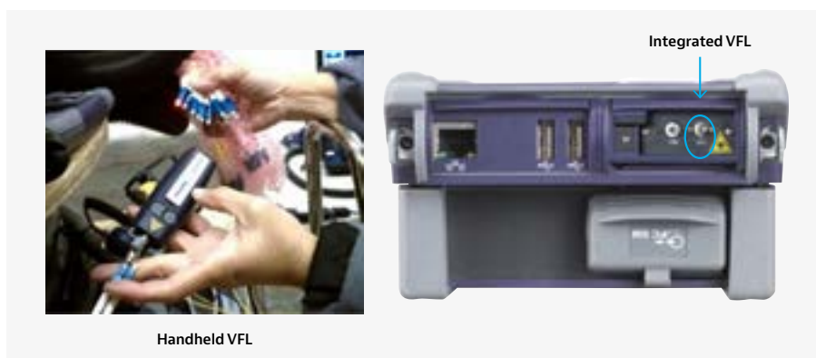
Figure 2: Fiber continuity test
