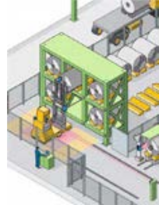
Fig. 4: Laser safety scanners create a curtain of laser light which senses the presence of persons or objects in potentially dangerous areas (SICK AG, Waldkirch).
