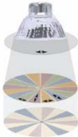
Figure 2: Structured polarisers exhibit regionally varying polarisation (orientation, spectral region)
