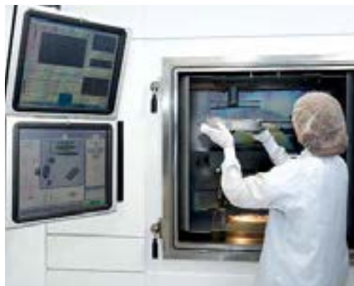
An ion-beam sputtering (IBS) coating chamber. Laser Components uses IBS coating technology to reach highest reflection and transmission values, from 248- to 3000-nm wavelength range (left). To reach the best possible results for high-quality laser optics, Laser Components controls the surface roughness by using white light interferometry (right).
