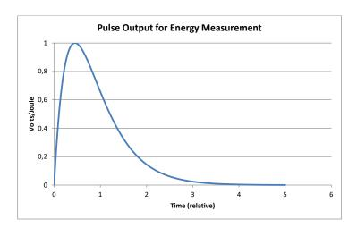
The amplitude of the pulse is the total energy in the detected heat pulse.
