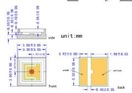
VD-0940C-020M-3A-2A0 with Substrate 3=<u>CuAg</u> and Package A=<u>2016</u> (unit: mm)
