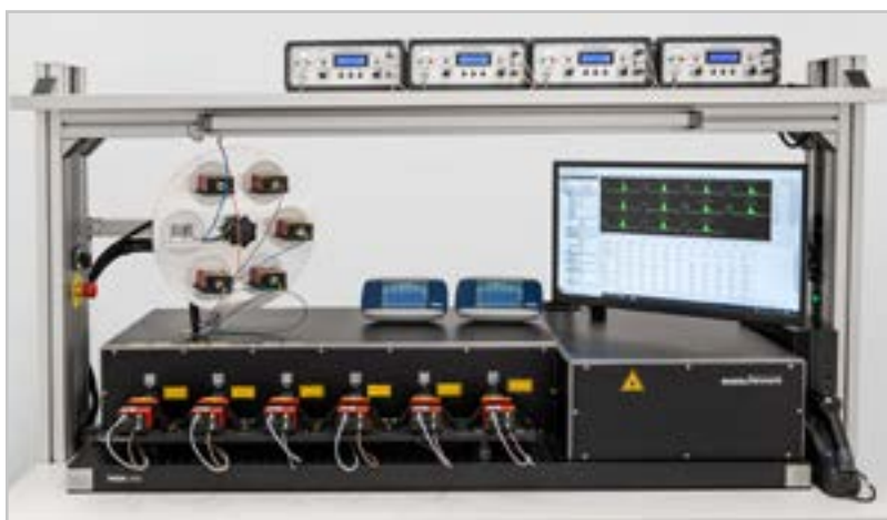
Figure 1: COUNT® test setup: fiber-coupled and free-space measurements
