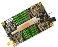
This NS series of fast-speed driver is designed to control NS series of solid state variable optic attenuators (VOA). The push-pull output design is especially suitable for driving capacitive VOA loads, assuring the fast response time both on rising and falling of attenuation. The driver can be operated by 0-5V signal to control the attenuation of VOA.
