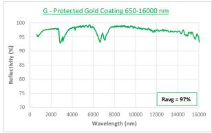
Note: Coatings meet Ravg requirement, but coating curves are for reference as R(\lambda may vary \pm 2% Detailed drawings and detailed coating curves are available on request.
