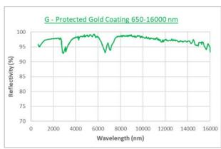
Coatings meet Ravg requirement, but coating curves are for reference as  $R(\lambda)$  may vary  $\pm~2\%$ Detailed drawings and detailed coating curves are available on request.
