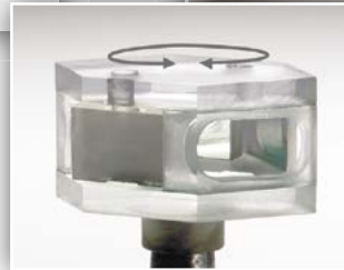
Monolithic scanning device: Designed to oscillate at a rate higher than 1KHz, while maintaining its stability and accuracy, this lightweight structure is balanced to reduce the moment of inertia about the pin axis.
