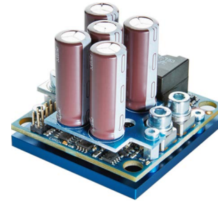
LDP-C driver with capacitor bank
