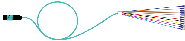
Figure 1: Example cable to be tested: Twelve fiber MPO breakout cable.
