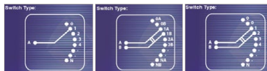
Figure 7 Single common (1C type), duplex (2D type), and dual parallel (2E type)
