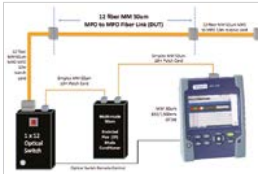
Figure 6. MPO Link Test Setup for faster testing
