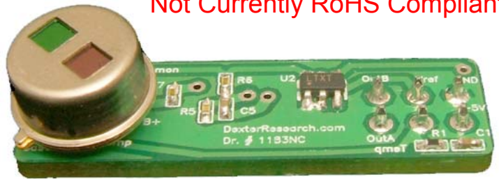
Miniature Dual Amplifier PCB w/ optional ST60 Dual (shown 3x actual size)
