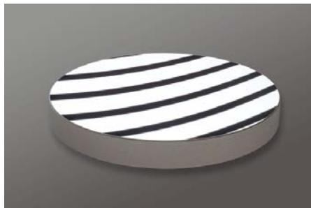
These mirrors are produced using a plasma-assisted reactive magnetron sputtering process, giving a high physical durability and temperature and humidity stability. Custom coating and substrate designs are available, allowing for optimisation within a specific range or coating on convex or concave substrates.
