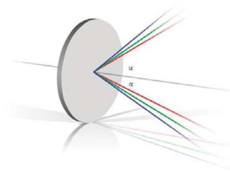
of the wavelengths produced. So-called triple mirrors are used for this purpose, for example in Nd:YAG laser systems that emit at the fundamental wavelength 1064nm and have harmonics at 532nm and 355nm, a
