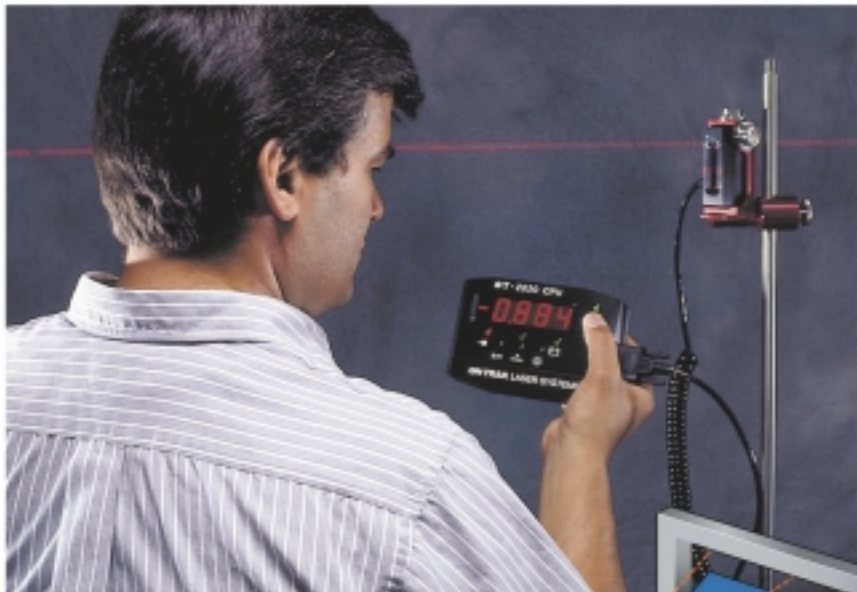
The OT-2020 Rotating Laser Target System measures flatness, squareness and straightness at distances up to 100 feet.
