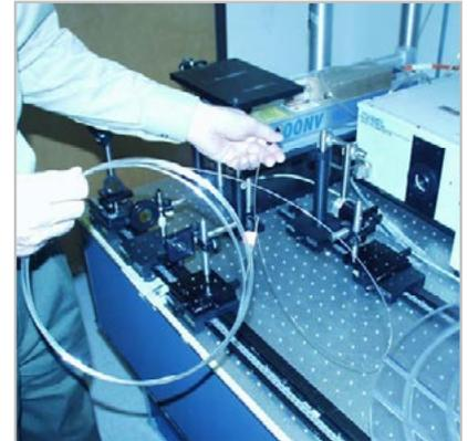
Figure 2: Hollow Silica Waveguide In Use
