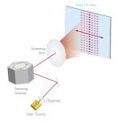
Scanning LIDAR illuminates a small part of the FOV at a time. The pulsed laser is scanned across the FOV (field of view) by using i.e. a rotating mirror. A rotating spin of 360° is doable. As little as a single photodetector (1 pixel or small array) captures the return.
