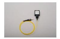
When the input optical power decreases, Signal Detect will change from high state to low state at a level (de-assert point) below the sensitivity. As the input optical power increases, Signal Detect will change back from low state to high state at assert point. The assert level is at least 1.0 dBm higher than the de-assert level.
