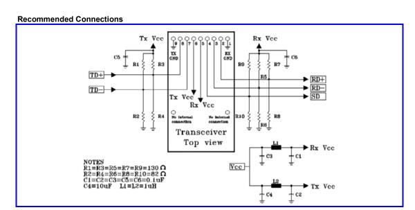
A connection circuit is recommended in the above diagram. The following guidelines are also recommended for designing the interface circuit:
