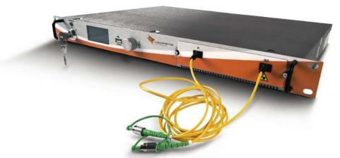
Our robust EDFA is appealing to this research and can offer up to 42dBm of saturated output power with a greater reliability. Furthermore, knowing that atomic cooling needs extremely stable laser with a narrow linewidth, we can offer a capability for a linewidth < 100kHz. Option of single mode fibre or polarisation maintaining fibre is available.
