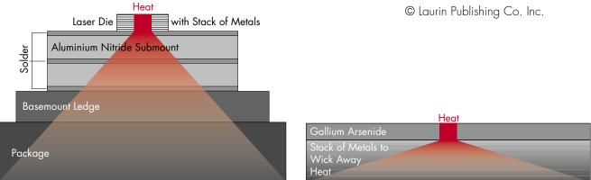
Fig. 1: Die, Submount and Housing
