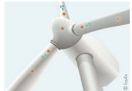
Schematic representation of the fos4Blade sensor platform inside a wind power plant.
