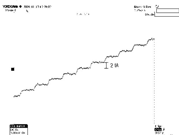
Both curves were recorded in the gain setting  $10^{12}$  V/A, filter setting 0.7 Hz, no external averaging (20 minutes warm-up before measurement).
