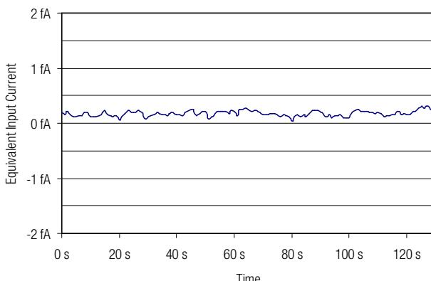
Both drift curves were recorded with shielded input in the gain setting  $10^{12}$  V/A, filter setting 0.1 Hz (20 minutes warm-up before measurement).
