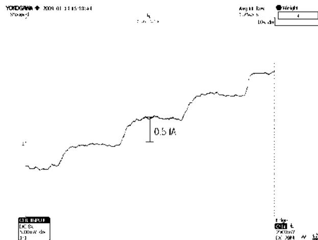
Both curves were recorded in the gain setting  $10^{13}$  V/A, filter setting 0.1 Hz (20 minutes warm-up before measurement).
