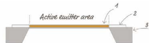
1 - Multi layer hot plate membrane containing NAC layer 2 - Bond pads 3 - Si frame and membrane
