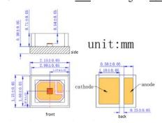
VD-0940C-010M-3A-2A0 with Substrate 3=CuAg and Package A=2016 (unit: mm)
