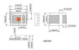
VD-0940C-010M-5H-2A0 with Substrate 5=NiFe and Package H=TO56 (unit: mm)
