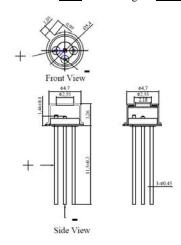
VD-0940C-010M-3W-2A0 with Substrate 3=<u>Cu/Ag</u> and Package Plastic Dip W=<u>0428</u> (unit: mm) (Remarks: Operating only in pulsed mode)
