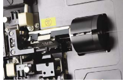
Precise alignment with resolution of 0.1 degree for 360 degree fiber rotation.
