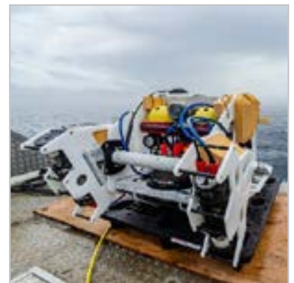
SeaVision™ mounted on unmanned underwater vehicle (Source: Kraken Robotics)
