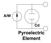
As capacitors they are high impedance devices and thus act as integrators of the voltage produced by their thermally induced current. Thus the voltage produced as a function of time is  $(v_c = \frac{1}{2} \int i dt)$ .
