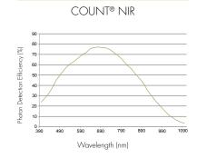
Typical photon detection efficiency
