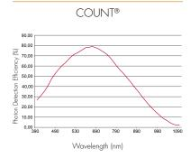
Typical photon detection efficiency
