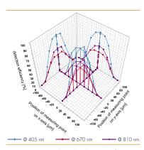
Measuring points along the detector surface
