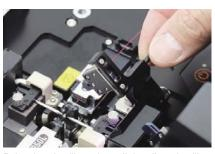
Releasing the fiber clamp links allow the fiber clamps to be placed without closing the canopy.
