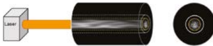
Transmission of Light in Multimode Fiber in Underfilled Conditions
