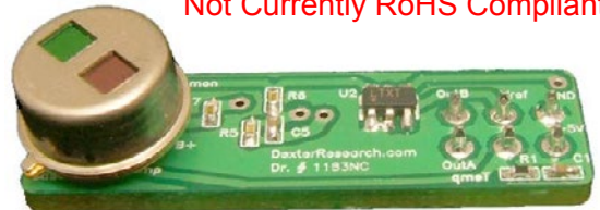
Miniature Dual Amplifier PCB w/ optional ST60 Dual (shown 3x actual size)
