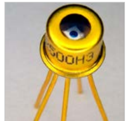
Figure 3: AC-coupled APD receiver in a 5-pin TO-46 housing
