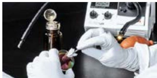
Cloth soaked in isopropanol cleans dielectric coated glass.
