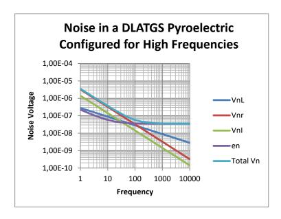
Notice that the noise in this configuration is dominated by the load resistor at the low frequencies and at the high frequencies by the loss tangent of the detector element and the JFETs voltage noise.
