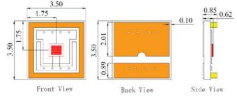
VD-0808I-002W-3E-2A0 (Substrate 3=Cu/Ag, Package E=7060) (unit: mm)
