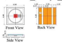
VD-0808I-007W-6K-2A0 with Substrate 6=Cu and Package K=T-mount (unit: mm)
