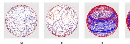
Figure 1. Poincaré sphere SOP traces for four different scrambling methods: (a) Discrete, (b) Typical Rayleigh or Triangle trace, (c) Tornado (fixed axis), and (d) Tornado (rotating axis).
